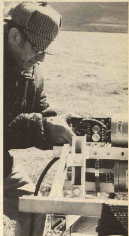
Charles Wyckoff loads film into one of the stereo 35-mm. cameras, in preparation for its first "splashdown" in Loch Ness. The stereo cameras would allow more precise measurements of any object photographed underwater, for sizes could be calculated using triangulation. (Photo: Dennis Meredith)
