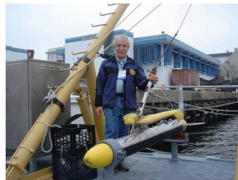
Martin Klein with a Klein multibeam side scan sonar. "We were proud that side scan was able to finally replace the old wire drag technology." (courtesy Martin Klein and the MIT Museum)
